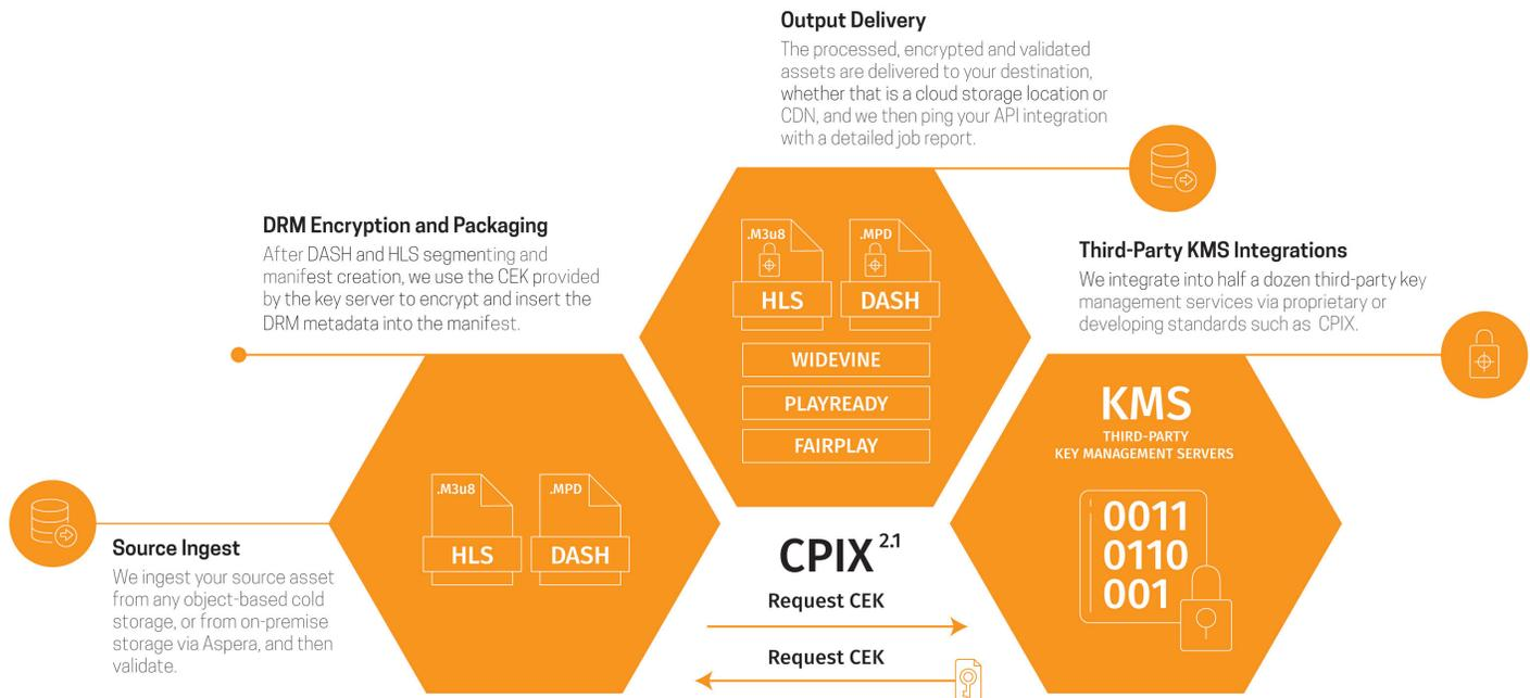
Transcoding and encryption in the cloud with Encoding.com simplifies the DRM workflow.
